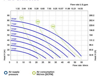
The curves and performance values refer to pumps with submerged suction and a free delivery outlet with water at 20°C. These data may vary according to the construction materials and hydraulic conditions.
